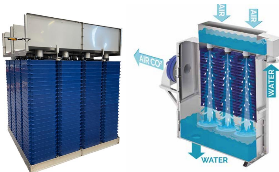
Figur 25: CO 2 –lufter for ras anlegg (Kilde: NP Innovation).
