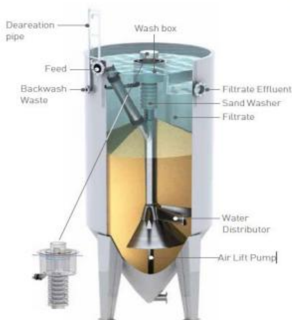
FIGUR 9.9 PRINSIPPSKISSE SANDFILTER
